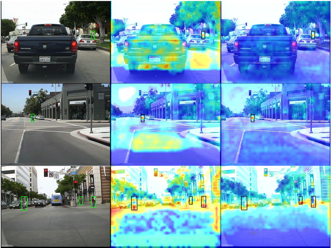
Figure 7: Qualitative analysis of the gating mechanism of our proposed AP 2 M on hard patterns of scale and occlusion. The 1 st is detection results of our AP 2 M presented by bounding boxes. Green or Black are true positives. The 2 nd and 3 rd column are “Spatial Heatmap” of GFFM at the 2 nd and 3 rd level, which determine the certain location where patterns are in need of further processing with more parameters by re-weighting them. The warmer the higher re-weight value in spatial heatmap \mathbf{H} \in (0, 1) .
